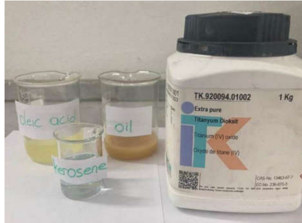
Figure 2. Oil flow visualization materials.
