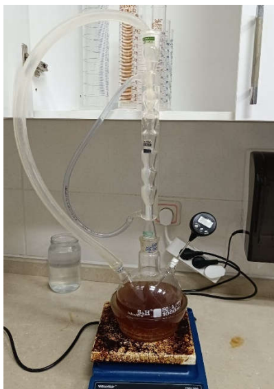
Figure 1. Transesterification reaction setup
