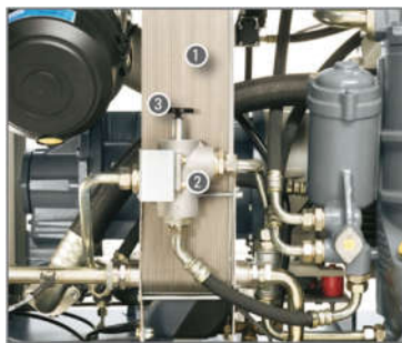
Figure 4. Plate heat exchanger inside the compressor [17]
