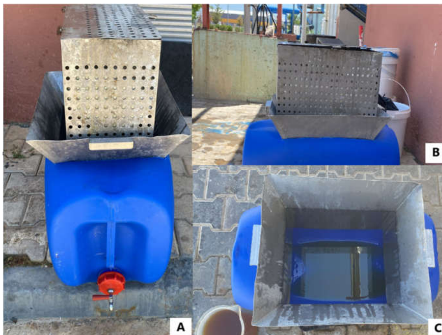
Figure 6. Filtration Process A: Filtration setup, B: Filter used for raw material filtration, C: Section where the liquid phase drains through filtration
