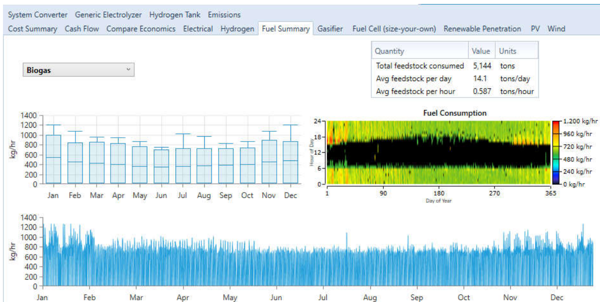
Figure 6. Biogas feedstock consumption patterns in microgrid systems
