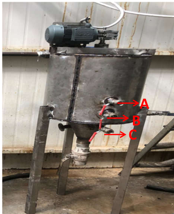
Figure 1. Reactor for the separation by density of fatty waste, Outlets A: The upper-phase sample collection valve, B: Non-settling particulates and water in the intermediate valve, C: Solids in the lower valve
