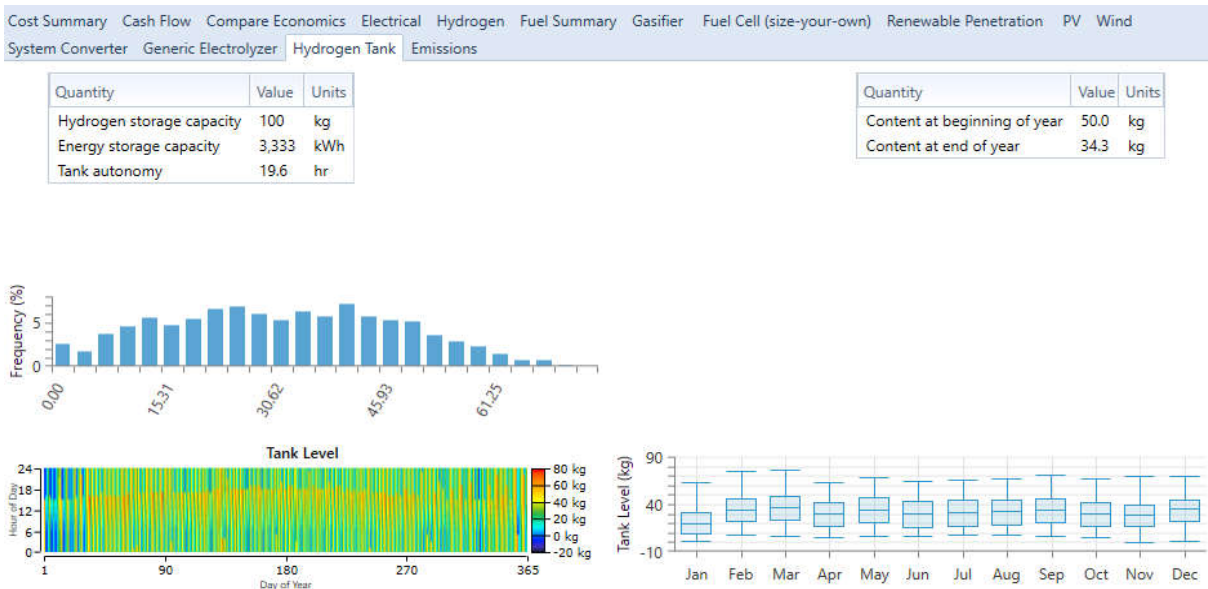
Figure 14. Hydrogen storage tank performance and utilization
