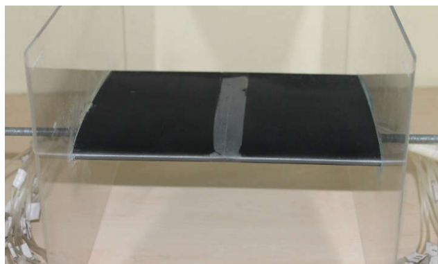
Figure 1. NACA 0012 airfoil prepared for pressure measurement experiment
