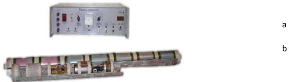
Fig. 4. General view of the device: a-control unit; b - three-phase influencer
