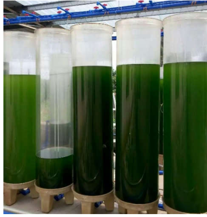
Figure5. Vertical Column Photobioreactor Example (Burgess, 2021)
